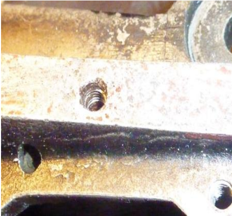
Typical of many sunken 'Helicoils'
